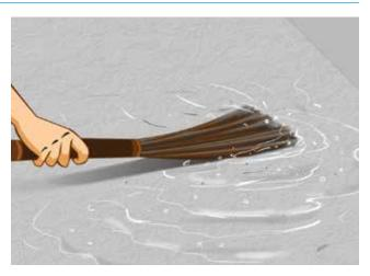
To ensure proper adhesion surface should prime with a single coat of Dr. Fixit Primeseal dilute with water in the ratio 2:1 and apply @ the rate of 8-10 Sq.m/L.
